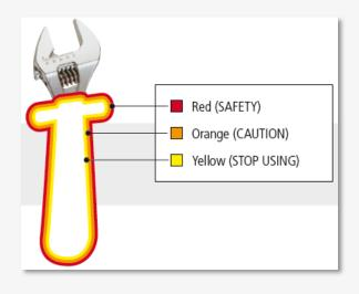
Every IREGA 1.000V adjustable wrench undergoes a HIGH VOLTAGE TEST, according to EN-60900 Standard, equivalent IEC-900, and consisting of a 10.000V charge for 10 seconds, after which there should be no damage to the handle.
