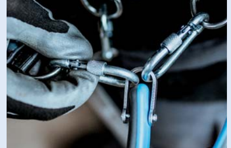
The carabiner on the lanyard has to be protected against opening using a lock ring.
