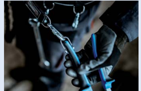
Correct attachment of the tool to the lanyard. Return the tool to the belt following the steps in reverse order.
