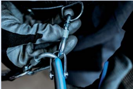
Before removing the tool from the belt, unscrew the lock ring on the carabiner on the belt.
