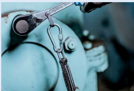
Use of ratchet. The ratchet does not have a button for switching sockets like a standard ratchet.
